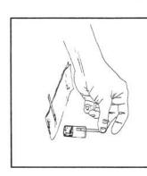
Dip one nitrite strip into sample for 2 or 3 seconds, remove, and place face up on paper towel.
