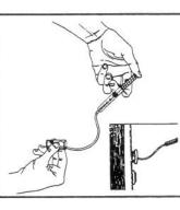
Using the syringe, draw coolant sample and dispense into the vial. (Sample should be below 110° F.)
